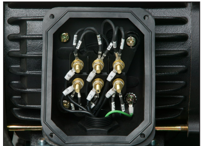
Figure 78. Model G0638 motor wiring (220V).
